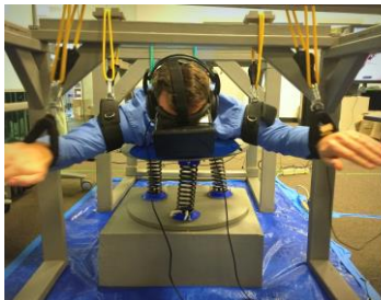
Figure 8. A user wearing an Oculus Rift, with their torso resting on a wooden base and their arms and legs suspended from the wooden frame, experiencing Prototype I during preliminary deployment.
