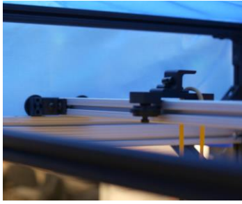
Figure 2. Horizontal sliders move in the XY plane as the user moves their arms to mimic a swimming gesture. The sliders are attached to resistance bands (in yellow), which are attached to user's arms and legs to simulate drag forces. Neoprene sleeve attachments are used to distribute forces uniformly on the user's limbs.
