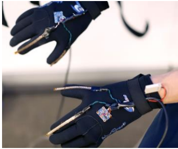
Figure 5. Gloves worn by the user. Each glove contains (a) an accelerometer, to track the user’s hand position, (b) flex sensors, to track finger movements, and (c) a Peltier module, to simulate temperature change.
