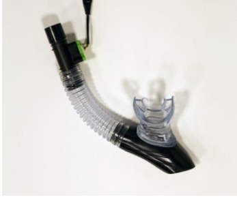
Figure 4. Mouth piece with Sensirion gas flow sensor [20] that measures the amount of air inhaled and exhaled by the user.
